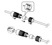
2. Connect the LAN connector (male) to the cable.
