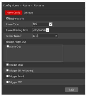
2. Enable the alarm to activate it and see the configuration parameters:
