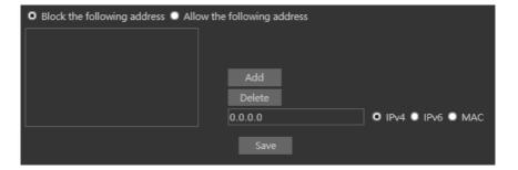
Enable the filtering you wish to activate. For the demonstration, we will enable both IP and MAC filtering, so the instructions below are true for both.
