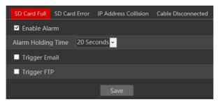
After enabling the alarm, choose the responses required from the camera in case the alarm will be active. After the setting is complete, click "Save".
