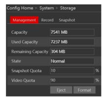
If it is the first time you are using the SD card with the camera or if the state is showing any value different than "Normal", you should click on "Format" before the SD card will be available for recording.
