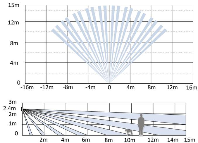
The detector will enter the walk test mode (3 minutes) after being enrolled.
