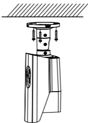
Figure 2-2 Fix the Camera to the Ceiling
