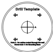
Figure 2-12 Drill Template of the Junction Box
