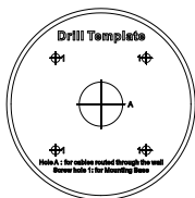
Figure 2-13 Drill Template of the Junction Box
