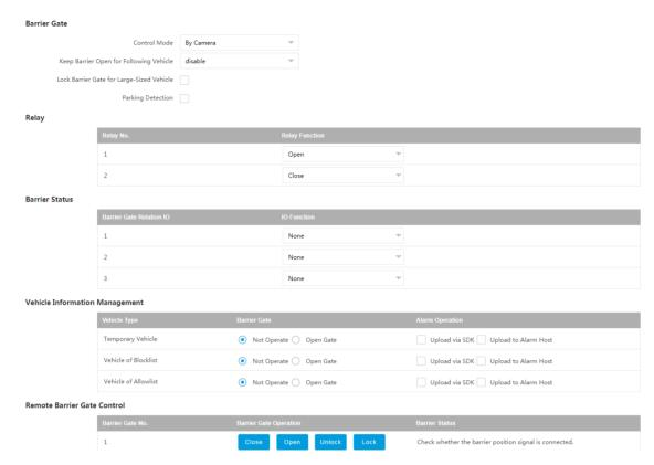
Figure 4-2 Control Barrier Gate
