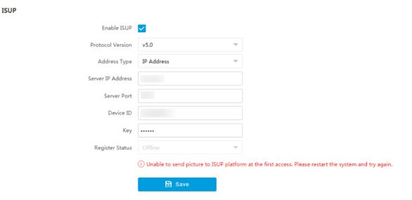
Figure 9-2 Connect to ISUP Platform
