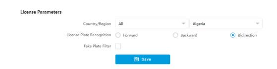
**Figure 3-5 Set License Plate Recognition Parameters**
