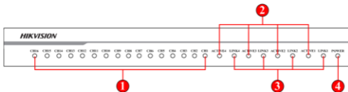
Figure 2.1 Rear Panel of DS-1H05-16R
