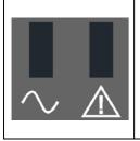
They are respectively inverter light and fault light from left to right.
