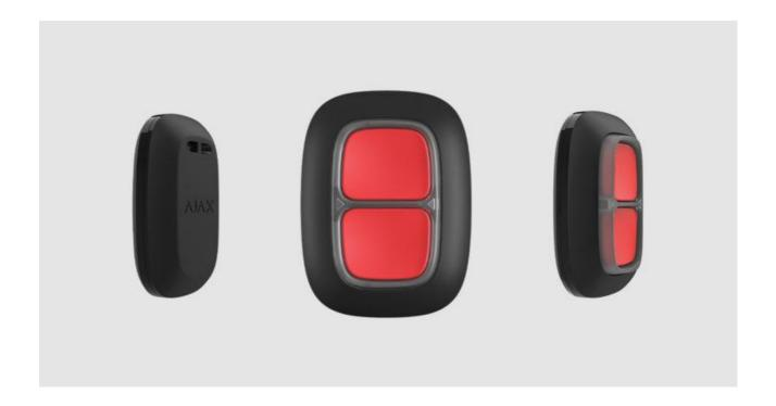
**DoubleButton** is a wireless hold-up device with advanced protection against accidental presses. The device communicates with a hub via the encrypted **Jeweller** radio protocol and compatible only with Ajax security systems. The line-of-sight communication range is up to 1300 meters. DoubleButton operates from the pre-installed battery up to 5 years.
