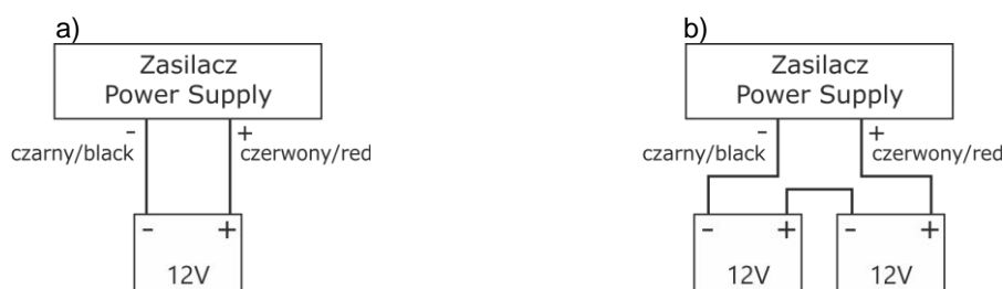
Fig. 4 Connecting batteries depending on voltage version of power supply: a) version 12V, b) version 24V,
