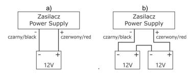
Fig. 4 Connecting batteries depending on voltage version of power supply: a) version 12V, b) version 24V,
