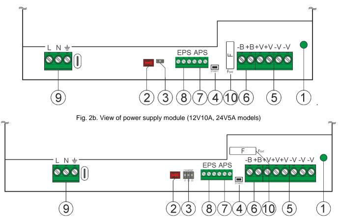
Fig. 2c. View of power supply module (12V20A, 24V10A models)
