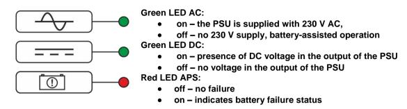
Moreover, PSU is equipped with LED indicating presence of voltage at PSU output, located on PCB of PSU module.
